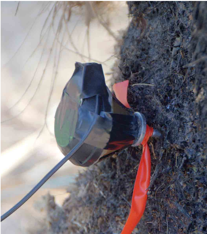
Figure 2. Acoustic sensor attached to a date palm stipe (stem).
