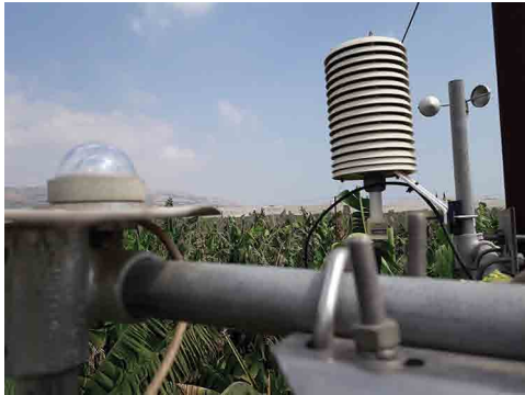
Figure 4. Climate sensors deployed above a banana plantation for computing atmospheric “dryness” and irrigation requirements. These include standard high-quality solar radiation (left), air temperature and humidity (middle) and wind-speed sensors.
