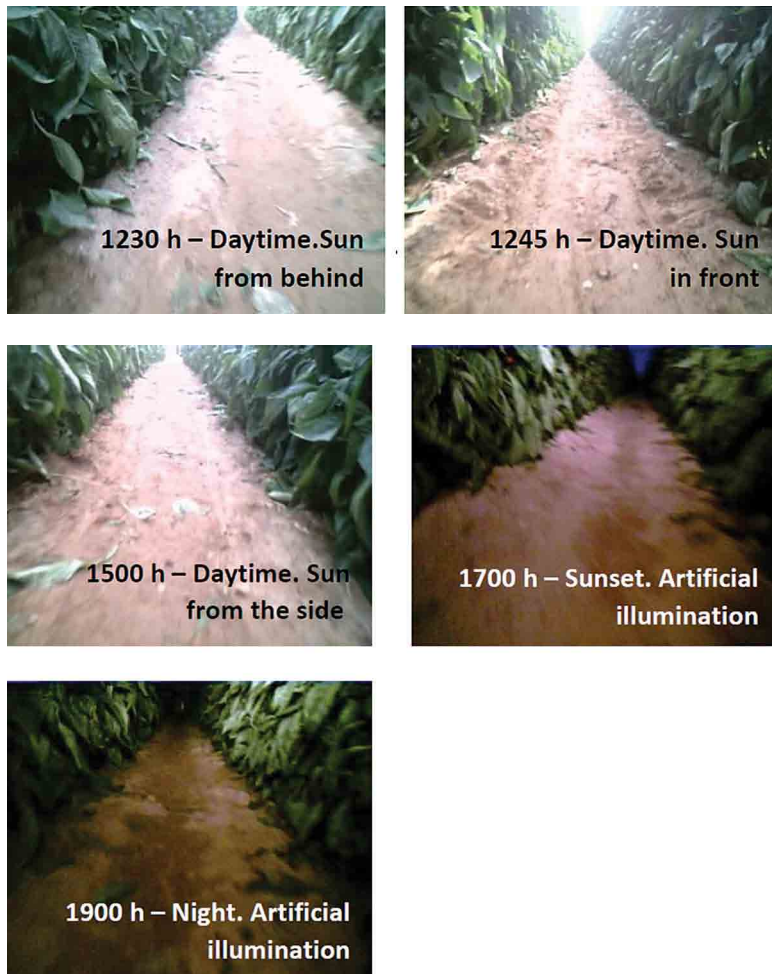
Figure 1. Pictures of an aisle between two pepper rows in a greenhouse taken from a robotic platform at five different times of day (Dar et al., 2011).
