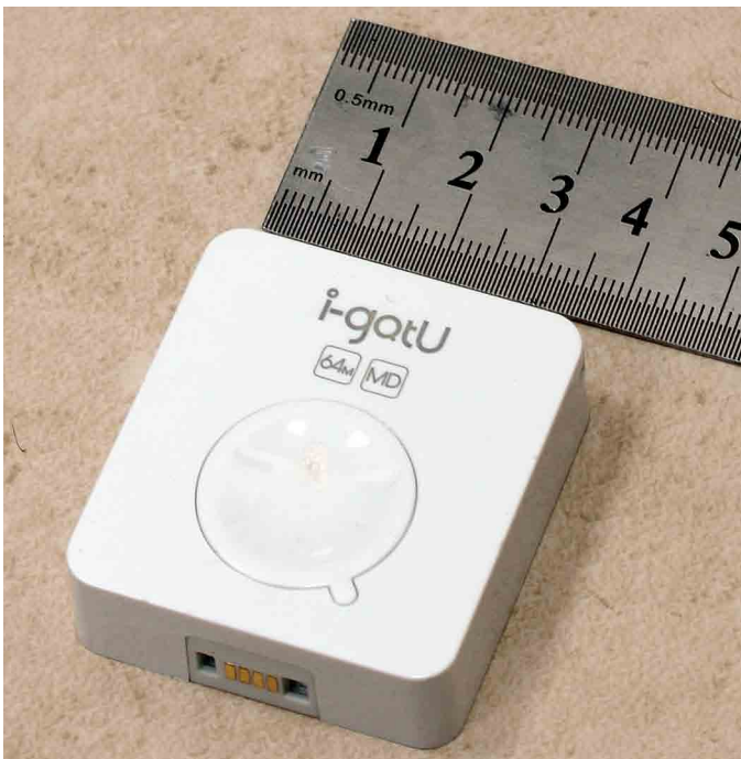
Figure 1. The general-purpose i-gotU GPS logger (Mobile Action Technology, New Taipei City, Taiwan) at the heart of the GPS collars used to map animal location on rangeland. The device weighs 37 g, contains a 750-mAh battery and can store 262,000 locations. A simple-to-use software interface enables the device to be programmed to operate with GPS fix intervals of 1 s to 1 h; the optional power-saving mode can be used for fix intervals \geq 7 s. Operation can be scheduled according to starting date and operating hours over a 24-h cycle, with a resolution of 1 h. A third-party external battery can be used in conjunction with the device's data/charging cable to greatly extend operating time.
