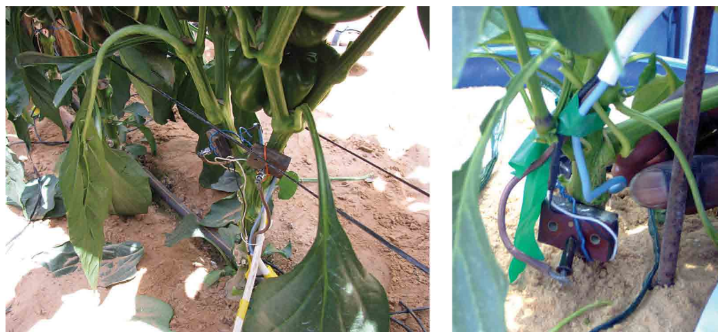
Figure 1. Sensors for measuring sap flow in pepper plants. The sensors were custom-built in Volcani’s workshop.
