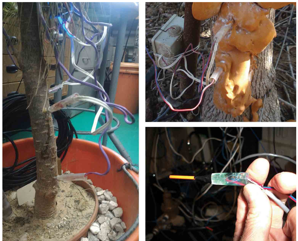
Figure 3. Sap flow sensors used in pine (left) and orchard trees (top right). The sensor assembly, built in our laboratory, is shown in the lower right.
