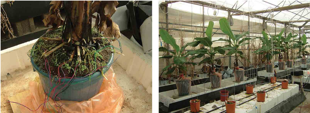
Figure 2. Banana plants with sap flow sensors built in our lab (left). Calibration of the banana sensors in a greenhouse using a series of banana plants on electronic scales (right).
